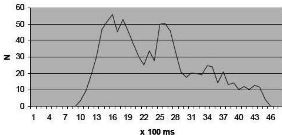
Fig. 3. Thrust force of drilling of cancellous bone.
